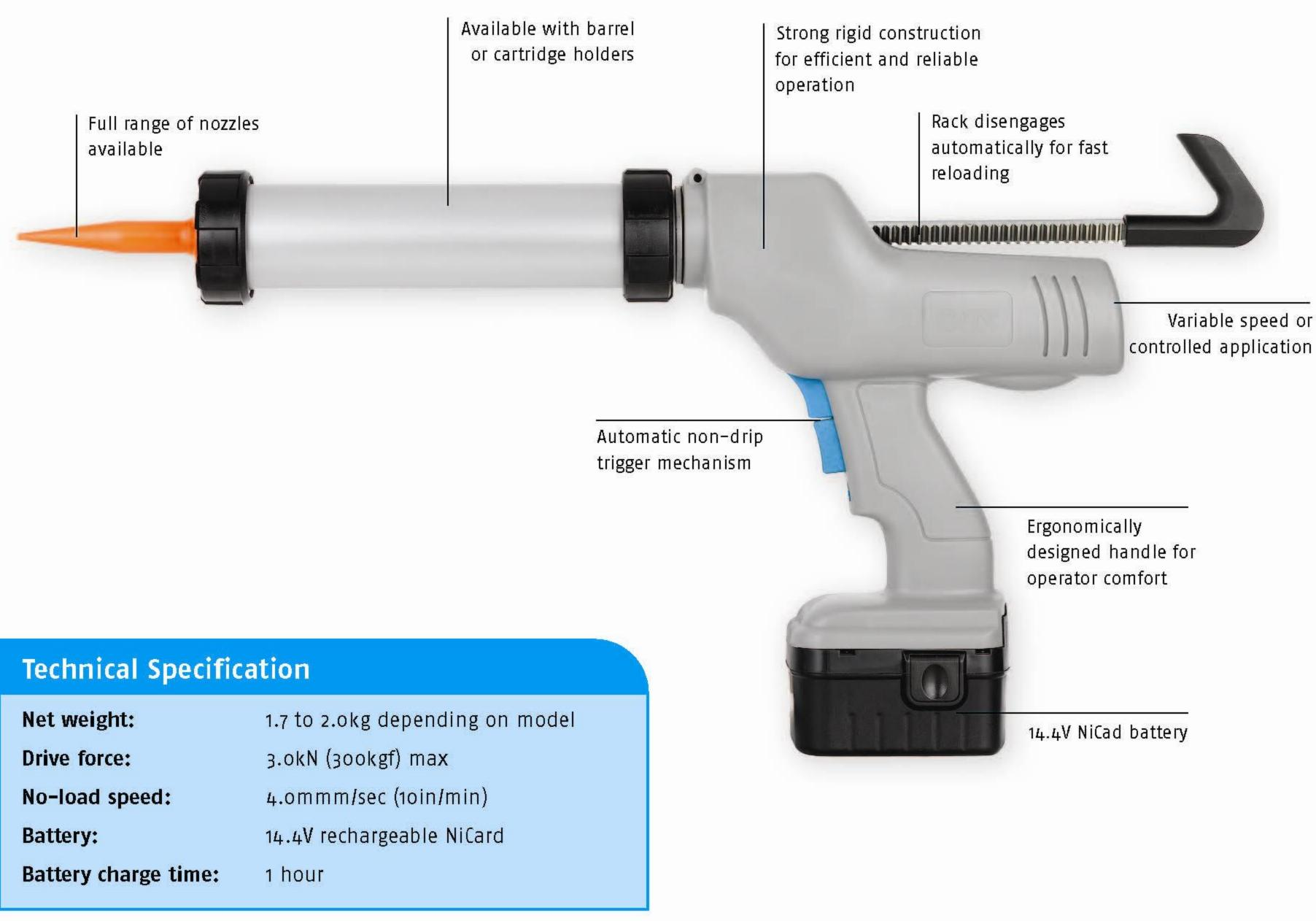
Models are supplied with charger and battery. Compatible with power supplies worldwide. A range of additional nozzles are also available.
